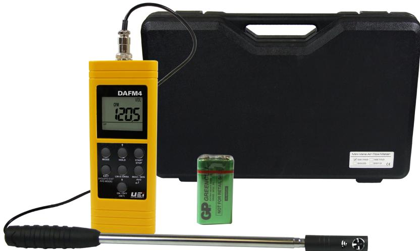
The DAFM4 is the tool for all your airflow measurement needs. With the DAFM4 you can directly capture air temperature, relative humidity, and air velocity. It also calculates wet-bulb temperature, dew point temperature, and air volume. Enter duct dimensions for live or timed average of air-flow in CFM (or CMM), or use the effective area of a grill for outlet volume measurements.
